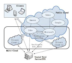
Fig. Cloud data storage architecture for Multi clouds
